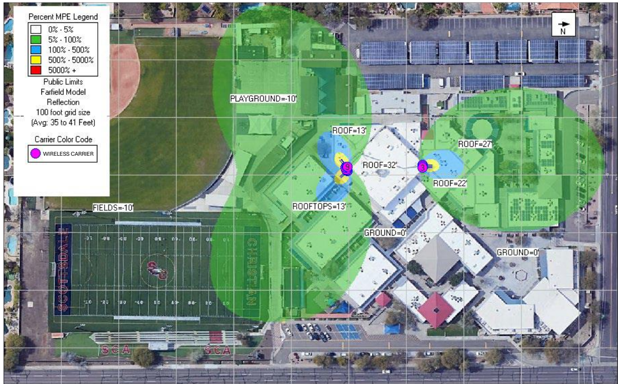
Fig. 5 – Predicted MPE as % of FCC General Population Limits (Ground Level)
