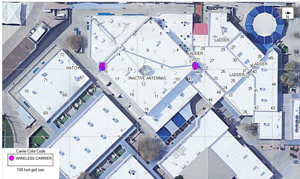
Fig. 3 – RF Measurement Locations on Rooftops
